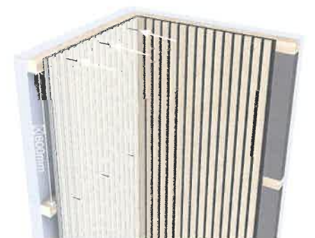
c. Install fiberglass wool or rock wool between the battens. absorption class: A
